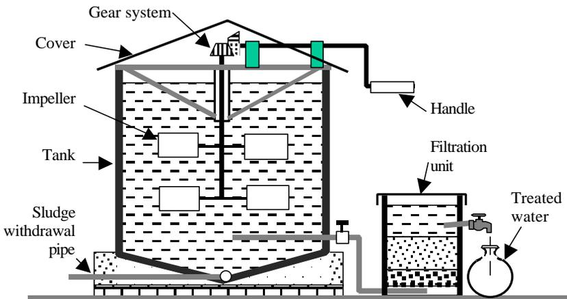
Figure 2 : DPHE-Danida Fill and Draw arsenic removal unit
